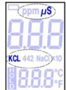
3. When the meter displays the desired selection. Release the 'HOLD/MODE' button.
